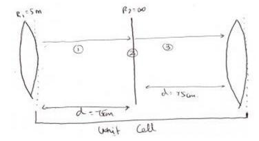
Ray path  $\rightarrow$  1- over a distance 'd' in air to the plane mirror; 2- plane mirror reflection; 3- over a distance 'd' in air to the spherical mirror
