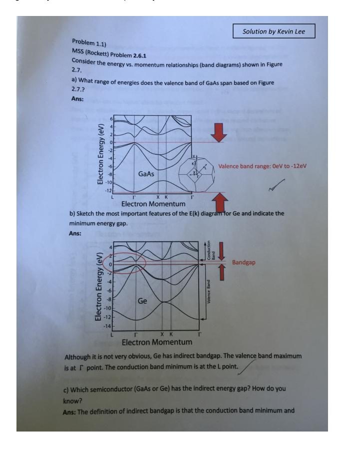
valence band maximum have the same momentum. From the above figures, we can easily see that Ge is an indirect bandgap semiconductor. The valence band maximum of Ge is at  $\Gamma$  point. The conduction band minimum is at the L point.
