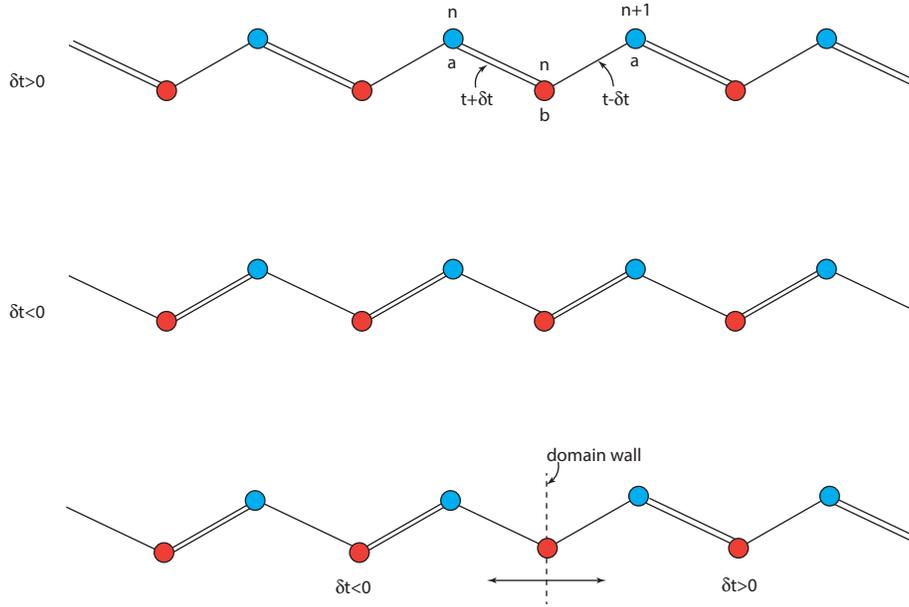
Figure 2: A polyacetylene chain that exhibits a non-trivial topological feature in its bandstructure.
