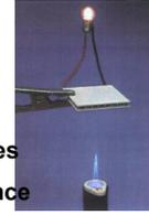
A thermoelectric cooler operated in reverse acts like a heat engine
