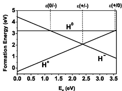
FIG. 15. Formation energies as a function of Fermi level for  $H^+$ ,  $H^0$ , and  $H^-$  (solid lines), and for a  $H_2$  molecule (dashed line) in GaN.  $E_F=0$  corresponds to the top of the valence band. The formation energy is referenced to the free  $H_2$  molecules.
