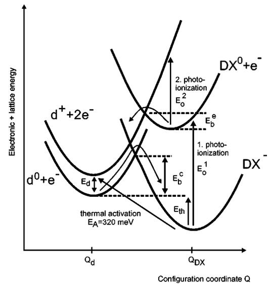
FIG. 12. Configuration coordinate diagram for a Si  $DX$  center in AlN, based on experimental information. From Ref. 139.
