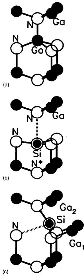
FIG. 11. Schematic illustration of the local environment around a silicon impurity in wurtzite AlN. (a) shows the ideal wurtzite lattice. (b) Illustrates the broken-bond  $DX$  configuration with bond breaking along the  $c$  axis (the so-called  $\gamma$ -BB center). (c) Illustrates another broken-bond configuration, with bond breaking along a different direction (the so-called  $\alpha$ -BB center). From Ref. 93.
