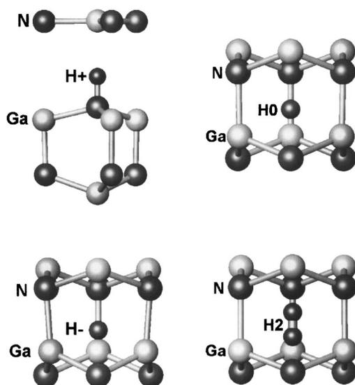
FIG. 14. Configurations of hydrogen in wurtzite GaN obtained from density-functional theory. The projection is orthographic, allowing lattice relaxations to be discerned.  $H^+$  resides at the bond center, while  $H^0$  and  $H^-$  are located at the center of the hexagonal channel. The  $H_2$  molecule also resides at the center of the channel, oriented along the  $c$  axis. From Ref. 176.
