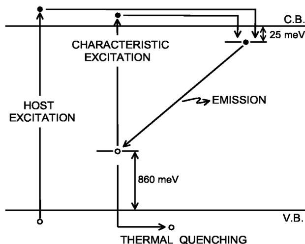
FIG. 7. Schematic illustration of the transition between a shallow donor and a deep acceptor that leads to the yellow luminescence in GaN. Ogino and Aoki<sup>95</sup> placed the deep acceptor level at 860 meV above the valence-band maximum. The calculated  $2-3-$  transition level of the gallium vacancy is located at 1.1 eV above the valence-band maximum.<sup>82</sup> From Ref. 95.
