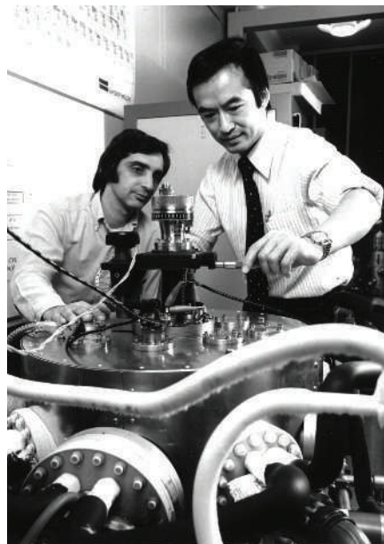
Figure 1 Al Cho (right) and Charles Radice working on an early MBE machine at Bell Labs in 1970. Although MBE was invented before the scanning tunnelling microscope and has had a major impact on both research and industry, it features much less prominently in accounts of the history of nanotechnology.
