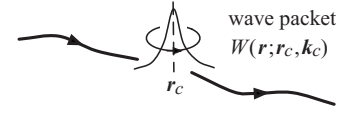
FIG. 10. The wave-packet description of a charge carrier whose center is (r_c, q_c) . A wave packet generally possesses two kinds of motion: the center-of-mass motion and the self-rotation around its center. From Xiao, Yao, et al. , 2006.
