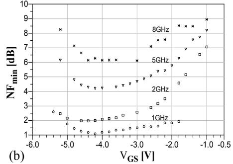
FIGURE 2. (a) Extracted  $f_T(V_{GS})$ , (b) measured  $NF_{min}$  at  $V_{DS}=2.75$  V.
