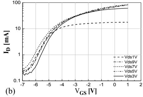
FIGURE 1. Measured (a)  $I_D(V_{DS})$ , drive  $V_{GS}/V=-6.5$  to  $-1.5$ , step 0.5 and (b)  $I_D(V_{GS})$ .
