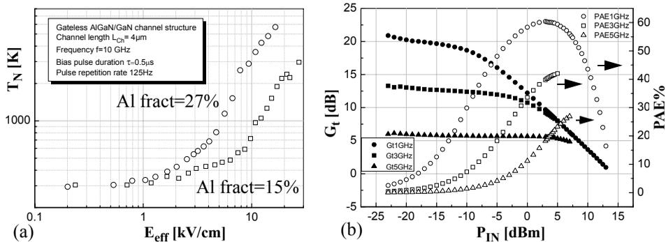
FIGURE 4. (a)  $T_N$  at  $f=10$  GHz, (b)  $G_t$  and PAE at  $V_{DS}=5$  V,  $V_{GS}=-5$  V,  $f$ [GHz]=1, 3, 5.
