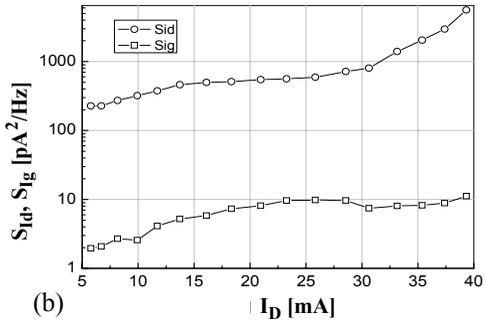
FIGURE 3. (a)  $NF_{min}$  at  $V_{DS}=2.75$  V,  $V_{GS}=-4.2$  V, (b) extracted  $S_{ID}$  and  $S_{IG}$  at  $V_{DS}=2.75$  V.
