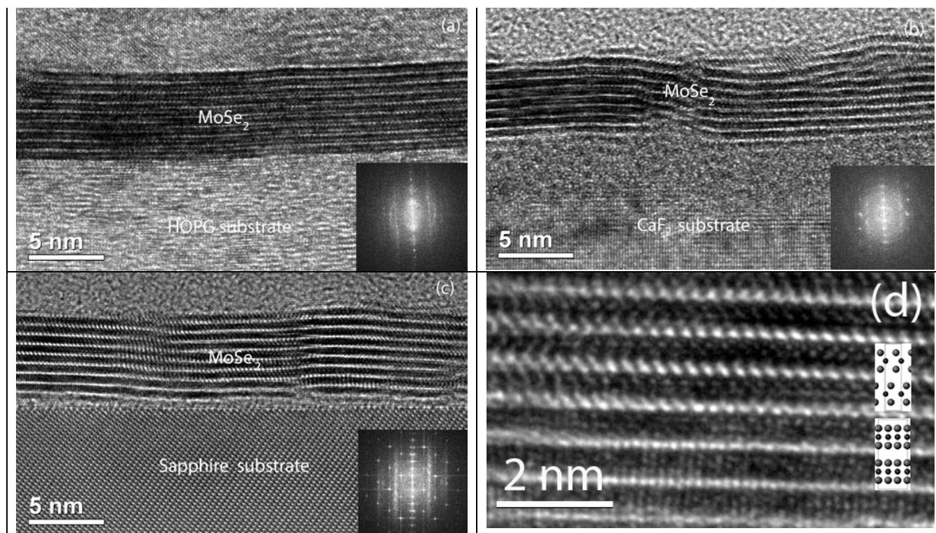
**Figure 1.** Typical cross-sectional HRTEM images of MoSe<sub>2</sub> on HOPG (a), CaF<sub>2</sub> (b) and Sapphire (c) substrates. Inserted are Fourier Transformations from the MoSe<sub>2</sub> layers and substrates. (d) is enlarged fragment of (c) to demonstrate turbo static disorder.
