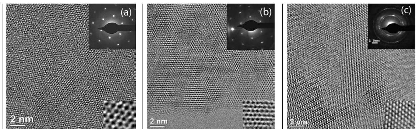
**Figure 2.** Plan view HRTEM images of MoSe<sub>2</sub> on HOPG (a), CaF<sub>2</sub> (b) and Sapphire (c). Inserted are corresponding electron diffraction patterns (top right corners) and enlarged fragments of the images (bottom right corners).
