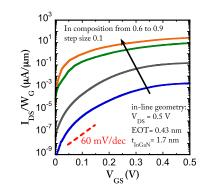
FIGURE 5. Transfer characteristics for inline TFET based on GaN/In<sub>x</sub>Ga<sub>1-x</sub>N/graded-InGaN/GaN heterojunction, with In mole fraction from 0.6 to 0.9. The calculated results are from TCAD simulations.
