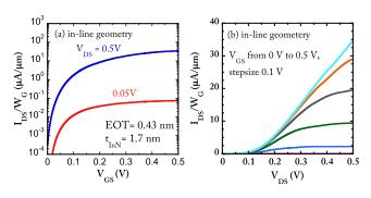
FIGURE 3. (a) Transfer and (b) output characteristics for an inline TFET based on an abrupt GaN/InN/GaN heterojunction.
