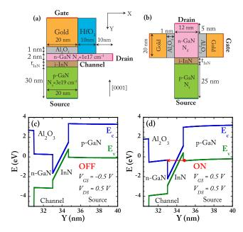
FIGURE 2. TFETs based on GaN/InN/GaN heterojunction. (a) Inline design, (b) sidewall-gated design, (c) OFF-state band diagram, and (d) ON-state band diagram for an inline TFET. The doping concentrations shown are the physical impurity concentrations.
