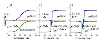
FIGURE 1. Computed band diagrams for (a) GaN homojunction, (b) staggered-gap GaN/InN/GaN heterojunction with 1.4-nm InN layer thickness, and (c) broken-gap GaN/InN/GaN heterojunction with 2.4-nm InN layer thickness.
