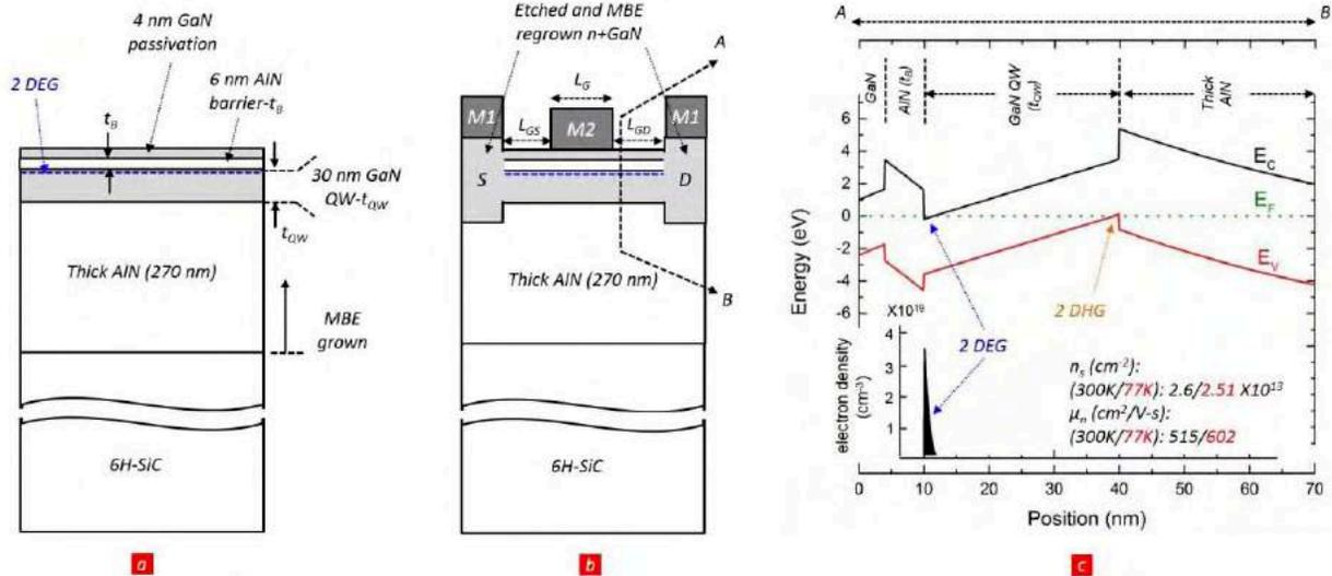
**Fig. 1.** a) Schematic of the strained AlN/GaN/AlN quantum well FET structure. b) Schematic of the processed device after MBE regrowth of n+ GaN source and drain regions, and ohmic and gate metal deposition (M1: Ti/Au, M2: Pd/Au). c) Energy band diagram of the QW showing the 2DEG channel at the top AlN/GaN hetero-interface, with the measured Hall-effect transport data in the inset.
