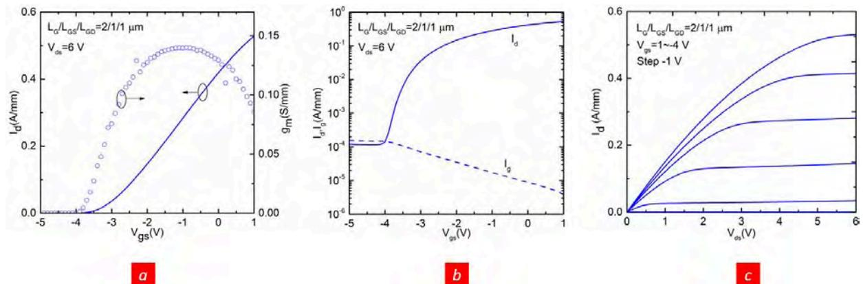
**Fig. 3.** Transistor characteristics for the 30 nm GaN strained quantum well FET with MBE regrown contacts. a) transfer curve at  $V_{ds}=6V$  b) semi-log transfer curve showing  $\sim 4$  orders on-off ratio, and c) DC output characteristics.
