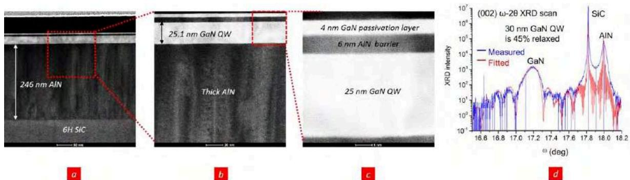
**Fig. 2.** Structural characterization of the strained GaN quantum well FETs. a-c) Z-contrast STEM analysis for a 25 nm GaN QW FET structure confirming abrupt hetero-interfaces between GaN and AlN. d) X-Ray diffraction spectra for 30 nm GaN QW sample showing the measured (blue) and theoretically calculated (red) curves that let us infer the thicknesses of the AlN and GaN layers. The GaN Quantum Well is found to be compressively strained as expected.
