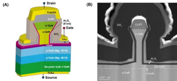
**Fig. 2.** (a) Schematic cross-section of the designed GaN TFET device. A buried  $n^+/p$  tunnel junction of large area is used to make a low-resistance ohmic contact to the buried p-type source layer. Cr/Pt metal is left over from the dry-wet process. (b) TEM cross-section image of the fabricated TFET. A golf-tee structure is formed due to Cr/Pt metal.
