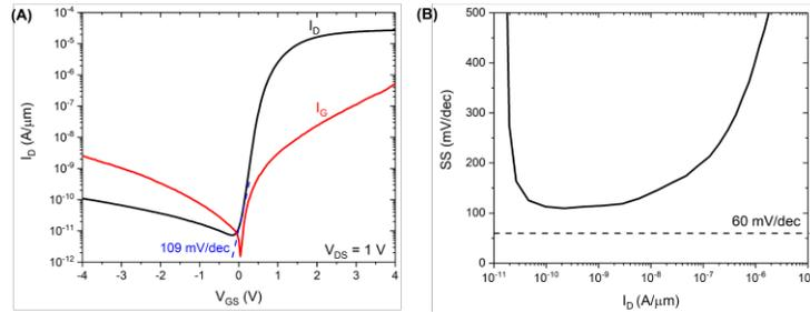
**Fig. 3.** (a) The measured transfer curve for 75nm wide GaN fin-TFET at 300 K. The minimum SS achieved is 109 mV/dec for an applied  $V_{DS}$  of 1 V. (b) The measured subthreshold swing versus drain current, extracted from Fig 3(a). While the SS is not below the thermal Boltzmann limit, the low SS is maintained over 2 orders of magnitude.
