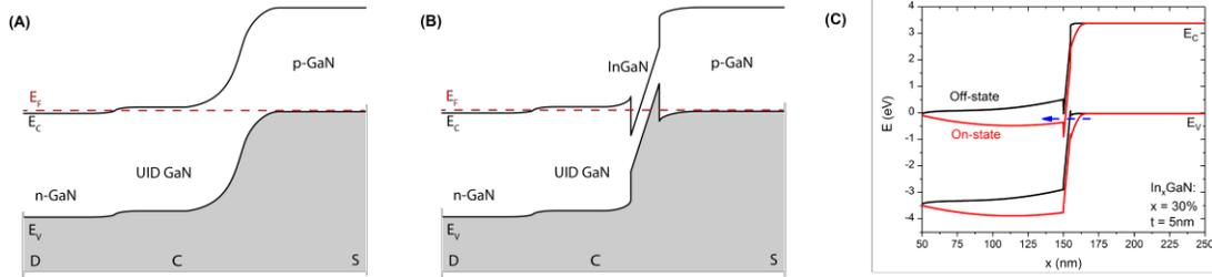
**Fig. 1.** (a) & (b) Energy band diagrams of GaN homo- and hetero- tunnel junctions respectively. Inclusion of InGaN reduces tunneling distance and increases the electric field. (c) Simulated energy band diagrams for the on and off state of a GaN heterojunction TFET
