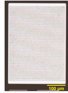
Fig. 3. Optical microscope image of the fabricated Ga 2 O 3 trench MIS-SBD with a fin-width of 3 \mu\text{m} .
