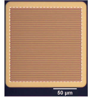
Fig. 3. Optical top view image of a fabricated device with a W_{fin} of 2 μm and a fin area ratio of 50%. The length of the fins is 150 μm. Central anode area within the dashed lines is used for current density calculation.
