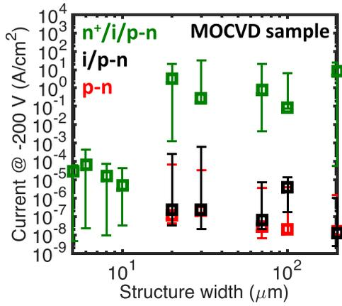
FIG. 5. Reverse leakage current at  $-200$  V vs. structure width for three types of diodes in the MOCVD sample. The error bars are generated based on the measurements of at least 3 devices with identical geometries. The sharp change in leakage near a width of  $10$ – $20$   $\mu\text{m}$  of the  $n^+/i/p$ -n diodes suggests that the buried p-GaN is sufficiently activated in small diodes ( $\leq 10$   $\mu\text{m}$ ) but not in large diodes ( $\geq 20$   $\mu\text{m}$ ).
