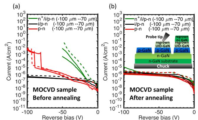
FIG. 2. Reverse I-V measurement of the circular diodes *w/o metal contacts* on the MOCVD sample: (a) before and (b) after the activation annealing at 725  $^\circ\text{C}$  for 30 min. The observed high leakage before annealing indicates that the p-GaN layer was re-passivated inside the MOCVD chamber.
