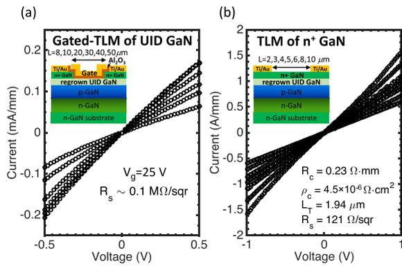
FIG. 3. TLM measurements on the MOCVD sample. (a) Gated-TLM I-V curves of the MOCVD-regrown UID GaN layer, measured at  $V_g = 25$  V. (b) TLM I-V curves of the MBE-regrown  $n^+$ -GaN layer. Insets show the schematic cross-section of the TLM structures. The gate dielectric in the gated-TLM structure is 30 nm of ALD  $Al_2O_3$ .
