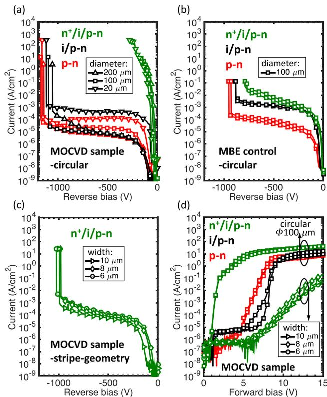
FIG. 4. Reverse and forward I-V characteristics of the three types of diodes. (a) Reverse I-V characteristics of circular diodes on the MOCVD sample. (b) Reverse I-V characteristics of circular diodes on the MBE control sample. (c) Reverse I-V characteristics of the  $n^+/i/p$ -n diodes with stripe-geometry on the MOCVD sample. (d) Forward I-V characteristics of the diodes on the MOCVD sample.
