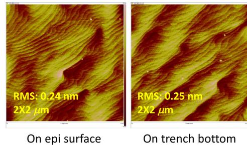
Fig. 2. AFM surface morphology of the MBE regrown UID-GaN channel on top of (left) epi surface (right) trench-bottom surface.
