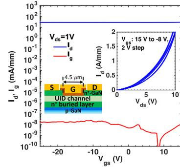
Fig. 5. Measured transfer and output  $I$ - $V$  characteristics of a planar test transistor fabricated on the same sample as the trench-MOSFETs with the  $n^+$  buried layer. Inset: schematic device cross section.
