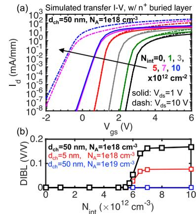
**Fig. 9.** (a) Simulated transfer  $I$ - $V$  characteristics in device *with* the  $n^+$  buried layer under different  $N_{\text{int}}$  values.  $d_{\text{int}} = 2 \text{ nm}$ . UID-GaN channel thickness:  $d_{\text{ch}} = 50 \text{ nm}$ . Acceptor concentration in p-GaN:  $N_A = 1 \times 10^{18} \text{ cm}^{-3}$ . (b) Extracted DIBL versus  $N_{\text{int}}$  under different  $d_{\text{ch}}$  and  $N_A$  values in p-GaN.
