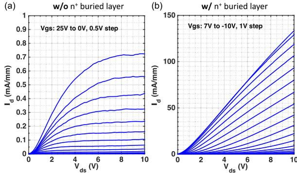
Fig. 4. Measured output  $I$ - $V$  characteristics of the trench-MOSFETs. (a) Without and (b) with the  $n^+$  buried layer. The device dimensions are the same, as described in Fig. 3.
