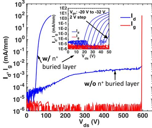
**Fig. 6.** Measured three-terminal breakdown characteristics of the regrown channel trench-MOSFETs;  $\sim 600$ -V BV and low drain leakage current are measured on the device without the  $n^+$  buried layer at  $V_{gs} = -15$  V. Soft breakdown behavior at  $\sim 130$  V limited by drain leakage current is observed for the device with the  $n^+$  buried layer. Inset:  $V_{gs}$  dependence of the drain leakage current in the device with the  $n^+$  buried layer.
