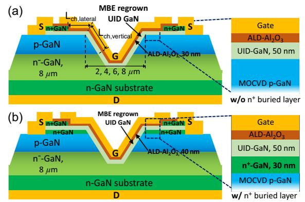
Fig. 1. Schematic cross section of two designs of the vertical GaN trench-MOSFETs incorporating MBE regrown UID-GaN channel. (a) Without and (b) with an  $n^+$ -GaN buried layer between the lateral part of the regrown UID-GaN channel and the p-GaN body.
