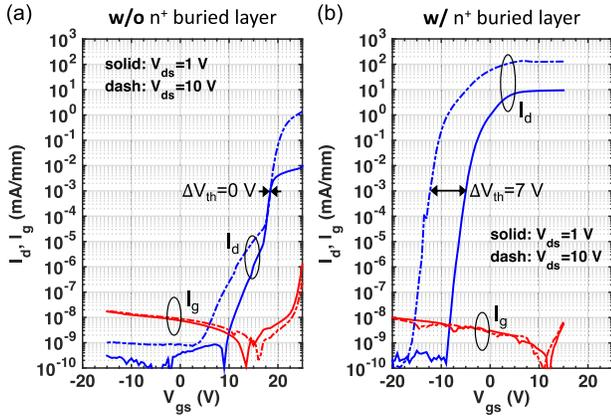
Fig. 3. Measured transfer  $I$ - $V$  characteristics of the trench-MOSFETs. (a) Without and (b) with the  $n^+$  buried layer. The representative device in (a) has a trench width of  $4 \mu\text{m}$  and  $L_{\text{ch,lateral}} = 3 \mu\text{m}$ . The representative device in (b) has a trench width of  $8 \mu\text{m}$  and  $L_{\text{ch,lateral}} = 1 \mu\text{m}$ .
