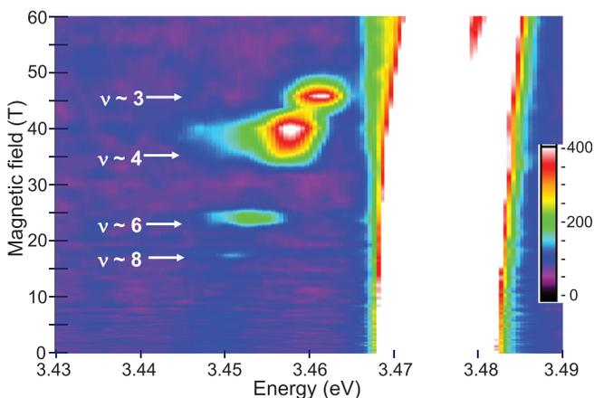
**FIG. 4.** PL measured up to 60 T. PL from the 2DEG brightens considerably at 17.5 T (as also shown in Figs. 2 and 3), 24 T, 39 T, and 46 T, which corresponds approximately to  $\nu \approx 8, 6, 4$ , and 3. Limited signal:noise precludes resolving the smaller intensity oscillations for  $B < 15$  T.
