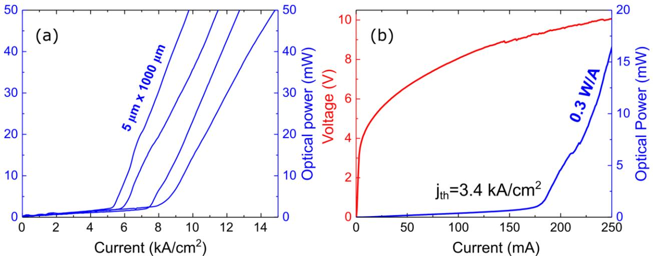
Figure 3. (a) Light-current characteristics of the inverted LDs under pulse operation. (b) Light-current-voltage characteristics of the best inverted LD from (a) under continuous wave operation.
