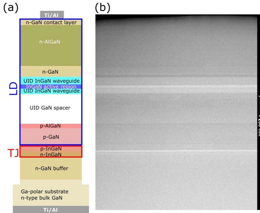
Figure 2. (a) Schematic image illustrating investigated laser diode layer structure with indicated tunnel junction (TJ) and flipped traditional laser diode layer stack (LD). (b) Transmission electron microscopy image of the grown structure corresponding to scheme presented in (a).
