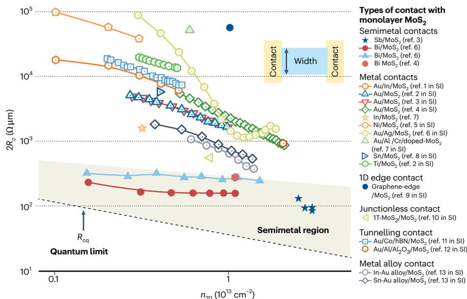
**Fig. 2 | Benchmarking of total contact resistance,  $2R_c$ , versus  $n_{2D}$  plot of experimental MoS<sub>2</sub> monolayer transistors.** Total contact resistance,  $2R_c$ , rather than  $R_c$ , is the appropriate parameter to compare with the ground-state ballistic quantum limit. Semimetal contacts currently provide the lowest contact resistances approaching the quantum limit. All measurements were
