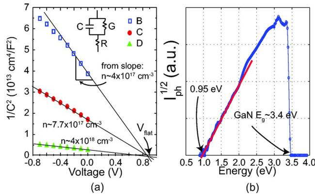
FIG. 2. (Color online) (a)  $C$ - $V$  measurements of InN/ $n$ -GaN diodes. (b) square root of photocurrent vs photon energy.
