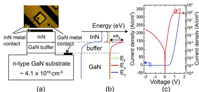
FIG. 1. (Color online) (a) The device structure of InN/*n*-GaN Schottky diode and (b) corresponding band diagram. (c) *I-V* measurement of the Schottky diode from structure A.
