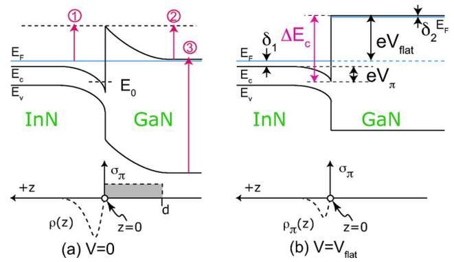
FIG. 3. (Color online) The band alignment and charge diagram of InN and  $n$ -GaN at (a) no bias and (b)  $V = V_{\text{flat}}$ . In the photocurrent spectroscopy, possible optically introduced transitions for the InN/GaN heterojunction are plotted in (a).
