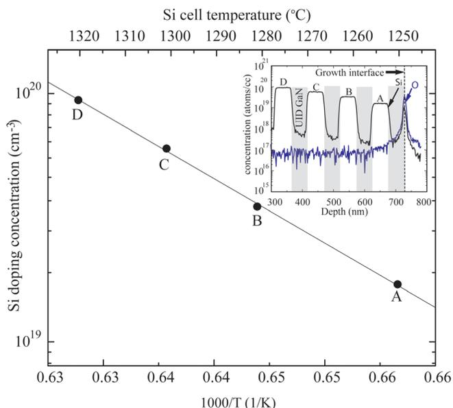
FIG. 1. Arrhenius plot of the Si concentration determined by SIMS, and the SIMS profile for Si and O concentration as a function of depth along growth direction is shown in the inset.
