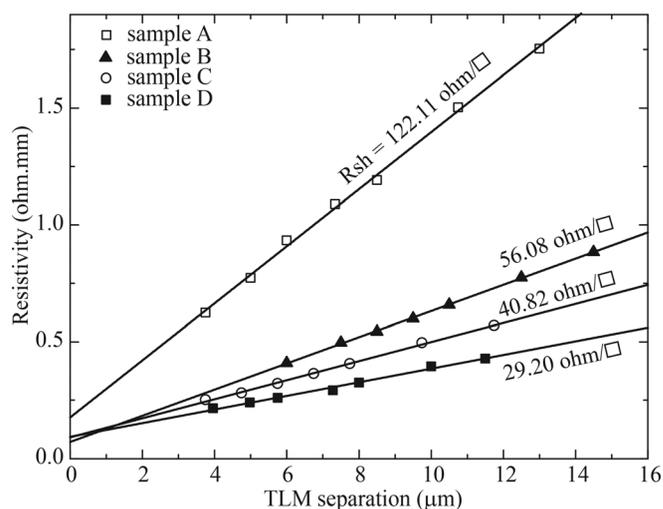
FIG. 3. Measured resistivity versus gap spacing plots obtained from TLM structures measured on samples grown using Si cell temperature of 1250 °C (A), 1280 °C (B), 1300 °C (C), and 1320 °C (D). The solid lines indicate linear fit to the experimental data points and extracted sheet resistance values are indicated for each sample.
