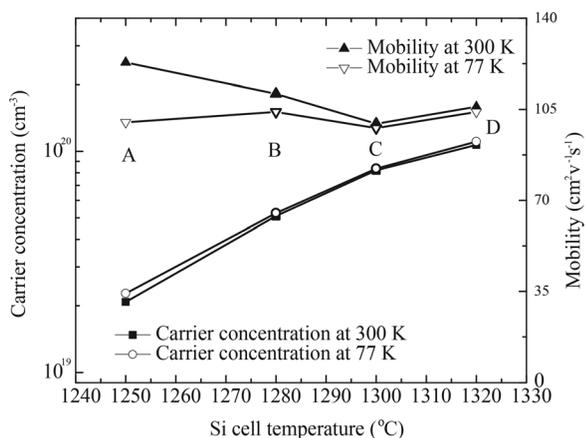
FIG. 2. Plot of carrier concentration and mobility of the  $n^+$  GaN samples obtained from Hall-effect measurements at room temperature (300 K) and 77 K as a function of corresponding Si cell temperature.
