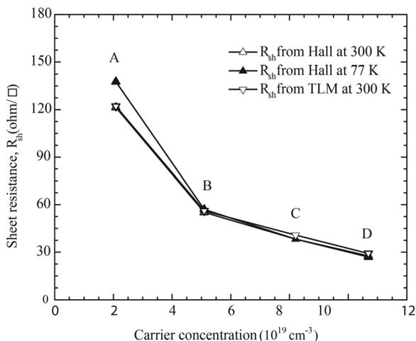
FIG. 4. sheet resistance versus carrier concentration plots obtained from room temperature TLM measurements and Hall measurements at room temperature (300 K) and 77 K.
