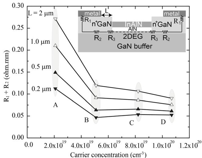
FIG. 6. Calculated values of  $R_1 + R_2$  as a function of carrier concentration for regrown  $n^+$  GaN ohmic contacts of a typical HEMT structure (inset). Four different cases of regrown  $n^+$  GaN similar to sample A, B, C, and D have been considered; for each case of regrown  $n^+$  GaN,  $L$  is chosen to have 4 different values of  $0.2$ ,  $0.5$ ,  $1$ , and  $2 \mu\text{m}$ .
