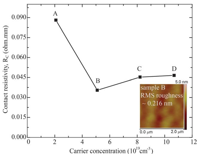
FIG. 5. Plot of contact resistivity versus room temperature carrier concentration of sample A, B, C and D.  $2 \mu\text{m}$  by  $2 \mu\text{m}$  AFM image of sample B with a smooth surface (rms roughness  $\sim 0.216 \text{nm}$ ) is shown in the inset.
