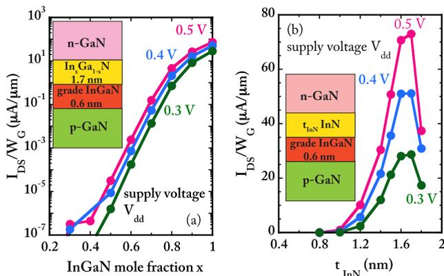
**FIGURE 6.** Inline TFET ON-current dependence on (a) InGaN interlayer In mole fraction and (b) InN layer thickness at supply voltages of 0.3, 0.4, and 0.5 V. Insets: corresponding heterojunction epitaxial structures. The calculated results shown in the figures are from TCAD simulations.
