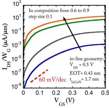
**FIGURE 5.** Transfer characteristics for inline TFET based on GaN/In<sub>x</sub>Ga<sub>1-x</sub>N/graded-InGaN/GaN heterojunction, with In mole fraction from 0.6 to 0.9. The calculated results are from TCAD simulations.
